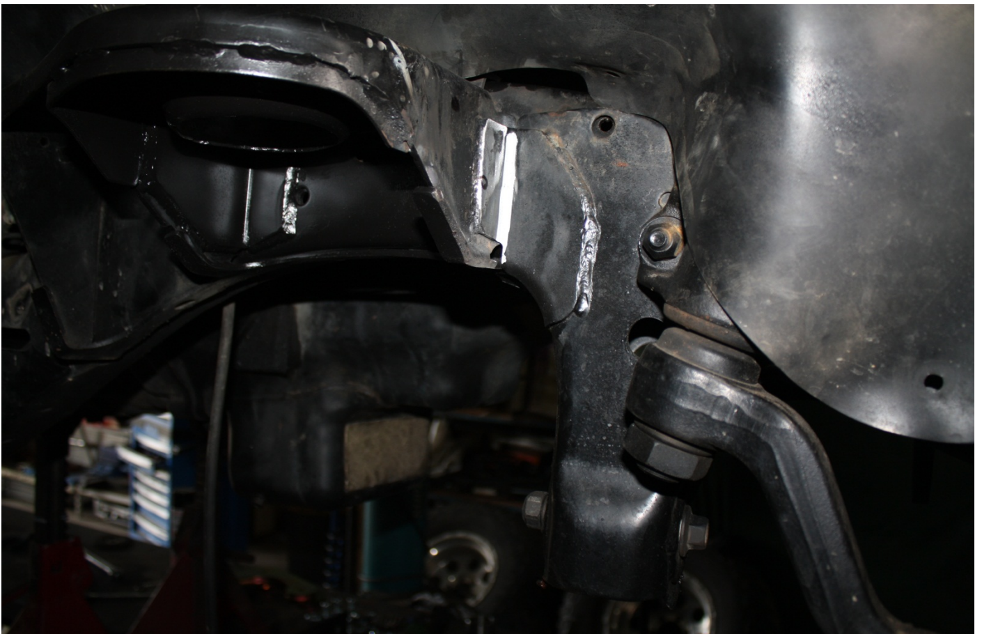
Figure 2: Factory Gusset Modification
