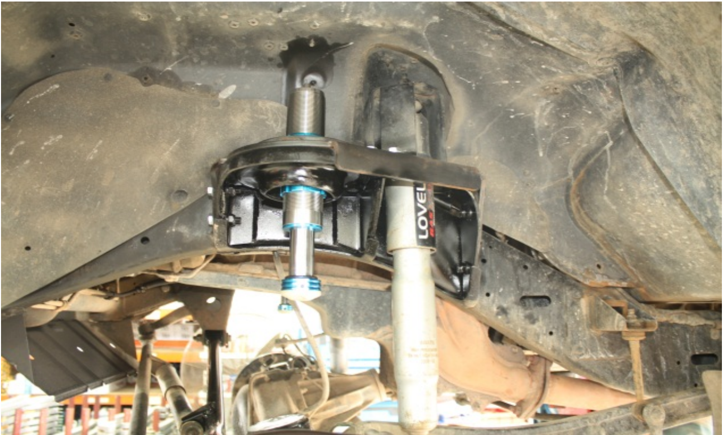
Figure 5: Correctly Fitted Bump Stop
