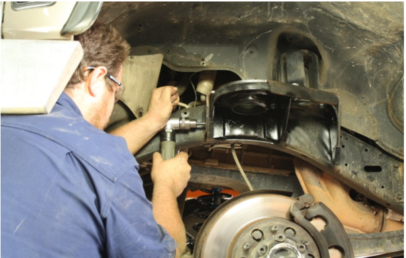
Figure 4: Drilling Of The Main Plate Holes
