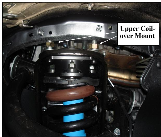
9. Now would be a good time to inspect the front coilovers for damage or fluid leakage. Replace if necessary.
