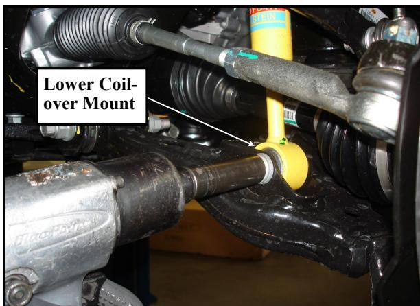
5. Support the lower control arm with a floor jack and remove the (2) lower knuckle mounting bolts.
