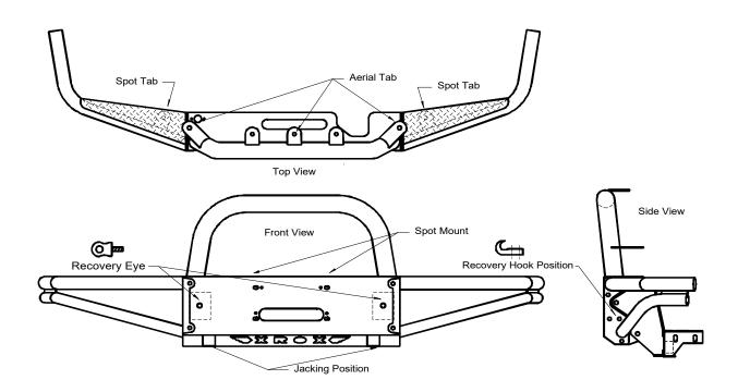
This bar has detachable side wings that can be replaced if damaged; plus 6 spot tab, 3 aerial tabs, 2 jacking positions, 2 recovery eye and 2 hook locations. (Recovery eyes & hooks are not provided in this kit). The bar has been developed to accept up to a 15,000Lb. Warn low mount winch.
