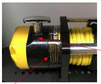
Split the second gearbox housing apart from the first housing, you only require a small gap in order to rotate the second housing
