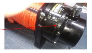
Rotate the freespool housing 90 degrees and replace and tighten all bolts this is normally the best position for a feet forward bar.
