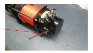
Once allen bolts are removed split the fresspool housing from the main gearbox housing as shown, you only require a gap of 1-2mm between the housings in order to rotate the freespool housing
