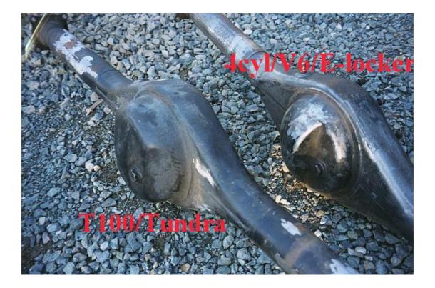
**4cyl 8" Differential:** All pre-'95 4-cylinder 4wd mini-trucks & 4Runners use the Toyota 8" 2-pinion differential front and rear (except turbo models). This is known as the "4cyl diff." This diff is by far the most common diff in older Toyotas. **See Pic Below**
