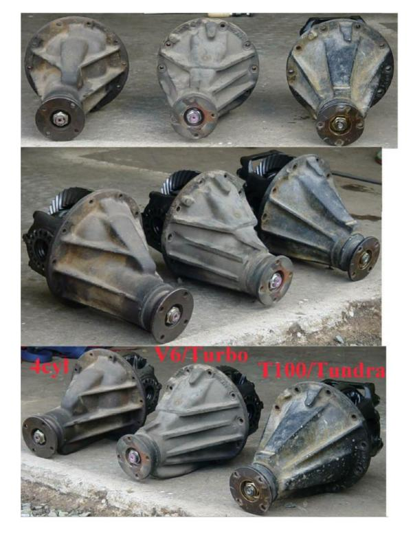
**Axle Housing Identification:** 4cyl/V6/E-locker has a dome-shaped cover. Diff uses 8mm studs with 12mm nuts. T100/Tundra/non-TRD Tacoma has deeper, blocky cover to accomodate the bearing truss. Diff uses 10mm studs with 14mm nuts. **See Pic Below**.
