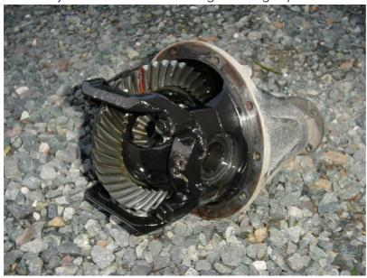
'07+ Tundra 5.4L V8, 10.5": The massive 10.5-inch Tundra rear ring gear, comparable to a 14-bolt or Dana 70. The big axles were offered with both 4.10 and 4.30 ring-and-pinions. Since most are found with the tow package, the majority will be 4.30:1. The
