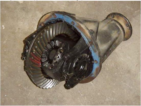
**V6/Turbo 8" Differential:** '86-95 4cyl Turbo and V6\* trucks and 4runners, and ALL '96+ 4Runners use the Toyota 8" 4-pinion differential in the rear. This diff is known as the "V6/Turbo diff." **See Pic Below**
