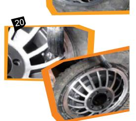
**18)**Reinfate the tyre to desired pressure: Under all circumstances, the tyre pressure should always be at least 5 psi less than the beadlock pressure and more difference is acceptable.
