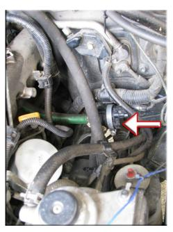
8. The pump draws very little current and can be directly connected into the wiring (white wire with red strip) as shown.
