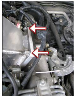
3. Loosen the 2 hose clamps holding the flexible hose between the turbo and the factory air intake cross member.
