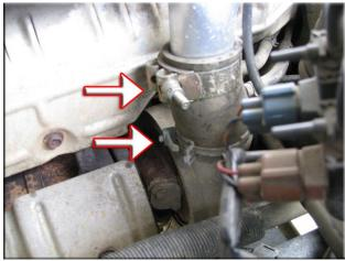
4. If fitted, undo the nuts from the exhaust gas recirculation valve flanges.
