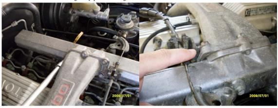
Remove the small pressure hose for boost compensation on the pipe.
