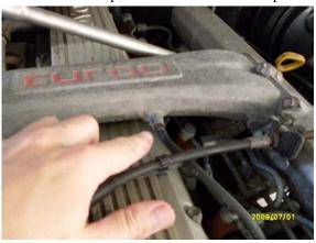
Loosen the clamp on the turbo hose's.
