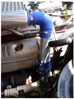
Connect the boost compensator hose and tight all clamps.
