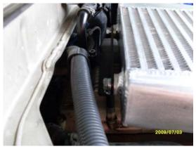
When the intercooler is in position, tighten all screws.
