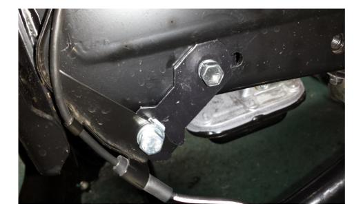
Refit original ABS bracket to new bracket as shown and tighten bolts to 18Nm
