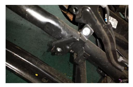
Remove original ABS wire mounting bracket from sway bar
