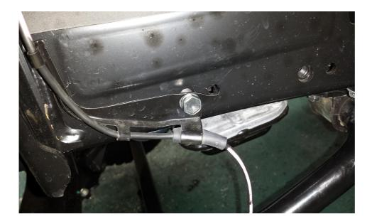
Remove original ABS bracket from chassis
