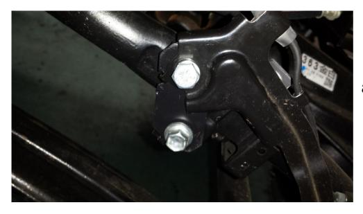
Fit original ABS bracket to the new location as shown and tighten bolts to 18Nm
